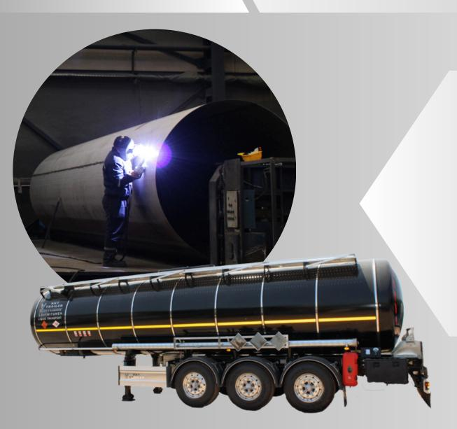
It is manufactured as a welded construction from high-strength stainless-steel material in accordance with ADR and the quality of the materials is presented with documented quality standards.
